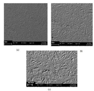
Figure 4.8 Microstructure of low carbon steel after hardening heat treatment (group C) by using SEM (a)  $500 \times (b) 1000x$  (c) 2000x magnification
