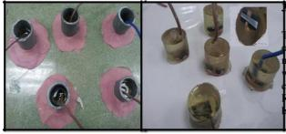
(a) (b) **Figures 3.5** cold mounting (a) pouring sample in pattern (b) sample after pouring
