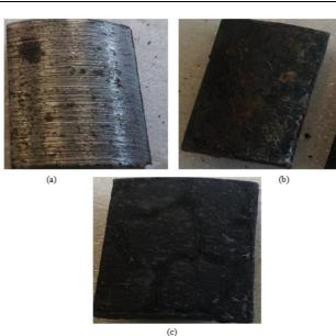
Figure 4.4 Un-corroded samples surface (a) Sample as-received (b) Sample annealed (c) Sample hardened
