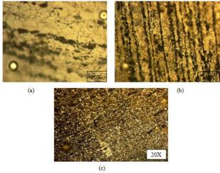
**Figure 4.5** Microstructure of low carbon steel without heat treatment by using OM of material (a) As received (b) after annealing (c) after hardening
