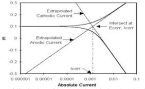
Figure 3.10 Classic Tafel extrapolation (Getting Started with Electrochemical Corrosion Measurement).
