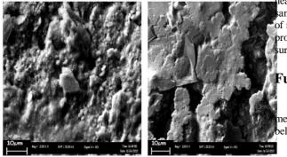
Figure 4.17 The SEM surface morphology of low carbon steel samples after hardening after soaking in 3.5 wt% NaCl solution (a) RH002 (b) RH003
