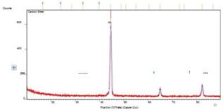
Figure 4.2 X-ray diffraction (XRD) analysis of low carbon steel
