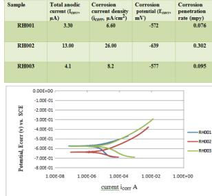
Figure 4.12 Tafel corrosion rate plot of group C in 3.5wt% NaCl solution
