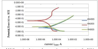
Figure 4.14 Comparison between three group's corrosion rates after 240 hour soaking in 3.5wt%NaCl solution
