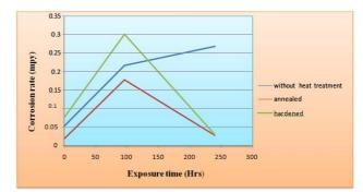
Figure 4.18 Relationship of corrosion behavior between three groups after soaking.
