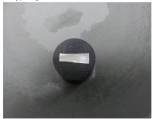
Figure 3.4 sample inside the poured by hot mounting
