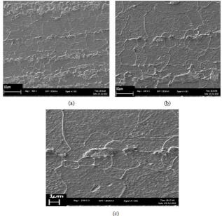
Figure 4.7 Microstructure of low carbon steel after annealing heat treatment (group B) by using SEM (a) 500 x (b) 1000 x (c) 2000 x magnification
