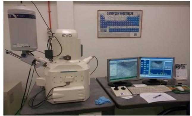
Figure 3.8 A Scanning Electron Microscope (SEM) (oxford, model7636)
