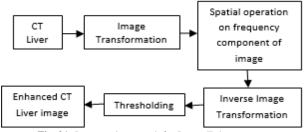
Fig. 21: Integrated approach for Image Enhancement.
