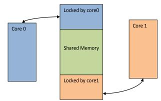
Fig. 2: Parallel Access to Different Memory Regions by Address-Sensitivity.
