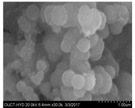
Fig. 1: SEM Image of Silica Particles.
