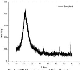
Fig. 2: XRD Characterization of Silica Particles.
