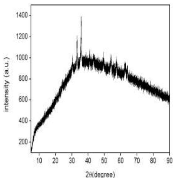
Fig: XRD graph for  $\alpha\text{-Fe}_2\text{O}_3$  Nanoparticles.
