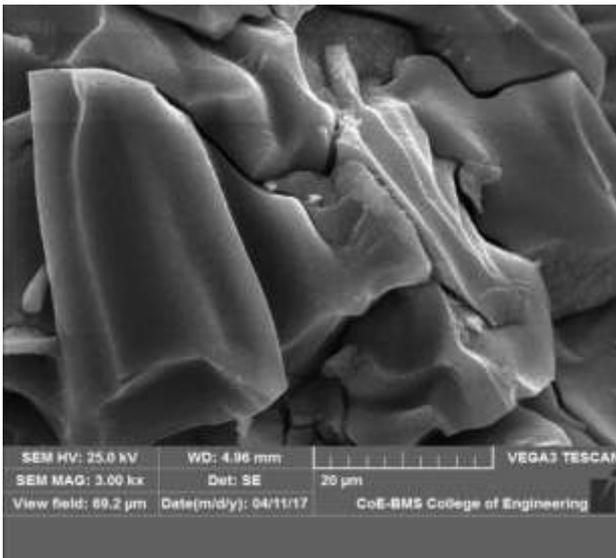
Fig: SEM images for  $\alpha$ -Fe<sub>2</sub>O<sub>3</sub> Nanoparticles.
