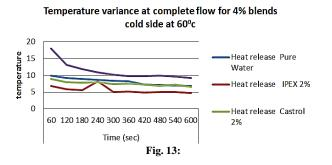
Above graph enhances the flow rate of different blends taken at 4% with temperature of 600c along cold side. Here the flow is complete which means liquid is circulated with maximum variance. The temperature is taken by calculating the mean  $\nabla t$ . the temperature is varied along with regular time interval of each 60sec
