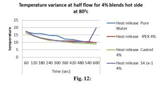
Above graph enhances the flow rate of different blends taken at 4% with temperature of 800c along hot side. Here the flow is half which means liquid is circulated with some stage variance. The temperature is taken by calculating the mean  $\nabla t$ . the temperature is varied along with regular time interval of each 60sec
