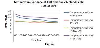
Above graph enhances the flow rate of different blends taken at 2% with temperature of 600c along cold side. Here the flow is half which means liquid is circulated with some stage variance. The temperature is taken by calculating the mean  $\nabla t$ . the temperature is varied along with regular time interval of each 60sec
