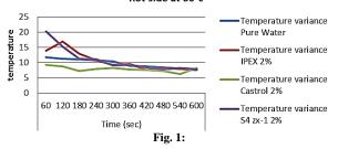
Above graph enhances the flow rate of different blends taken at 2% with temperature of 600c along hot side. Here the flow is complete which means liquid is circulated with maximum variance. The temperature is taken by calculating the mean  $\nabla t$ . the temperature is varied along with regular time interval of each 60sec
