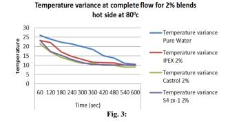
Above graph enhances the flow rate of different blends taken at 2% with temperature of 800c along hot side. Here the flow is complete which means liquid is circulated with maximum variance. The temperature is taken by calculating the mean  $\nabla t$ . the temperature is varied along with regular time interval of each 60sec
