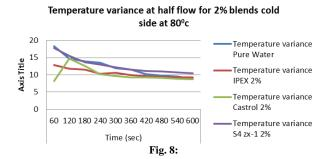
Above graph enhances the flow rate of different blends taken at 2% with temperature of 800c along cold side. Here the flow is half which means liquid is circulated with some stage variance. The temperature is taken by calculating the mean  $\nabla t$ . the temperature is varied along with regular time interval of each 60sec Temperature variance for all fluids with 4% blends along hot side:
