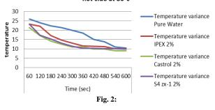
Above graph enhances the flow rate of different blends taken at 2% with temperature of 600c along hot side. Here the flow is half which means liquid is circulated with some stage variance. The temperature is taken by calculating the mean  $\nabla t$ . the temperature is varied along with regular time interval of each 60sec
