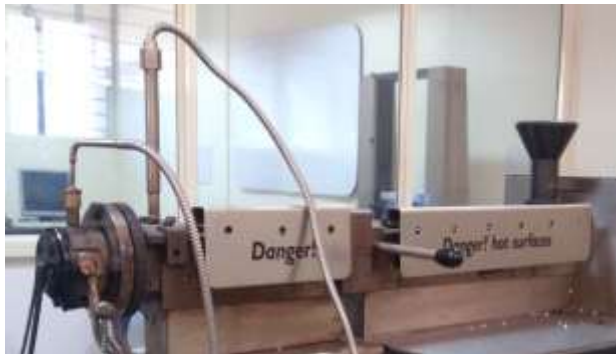
Fig 5: Extrusion process setup
