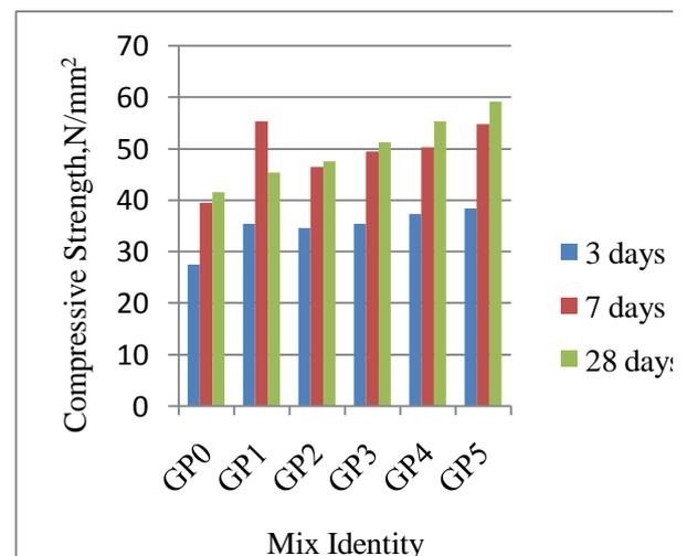
**Fig 1:** Compressive strength variation of FRGPC
