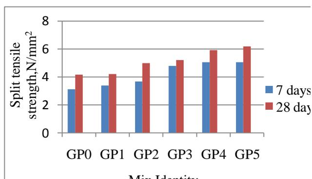
Fig 2: Split tensile strength variation of FRGPC
