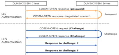
Figure 1: Authentication method of DLMS/COSEM
