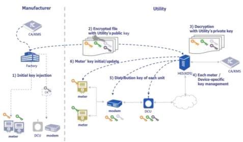
Figure 3: Design of Key distribute system for Smart metering
