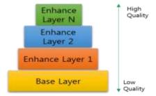
Fig. 4: Scalable Video Coding Conceptual diagram
