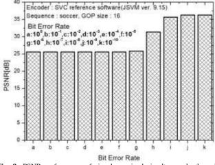
Fig. 9: PSNR performance of signals received simultaneously through VLC and sound communication dual transmission
