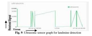
As shown in figure. 9, graph is between received signal delay and time. In the graph, there is absurdly high values of more than 2000cm which depicts the scattering of wave by sand. It also, at certain time, gives a finite value of 2 cm which depicts that a metal surface is found. Transition from finite to high value is also shown which explains the change of surface texture.
