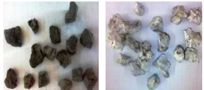
(a) Steel slag aggregates before weathering process (b) Formation of thin film of calcite on slag aggregates after undergoing weathering process
