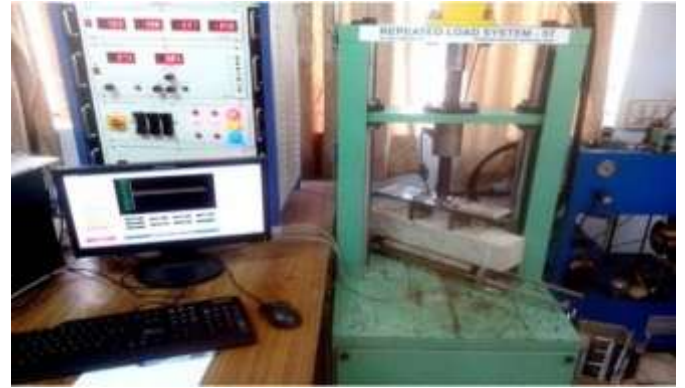
Fig. 2. Repeated load testing set up.
