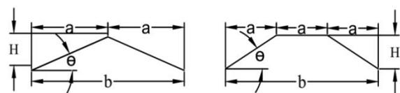
**Fig 1:** Typical cross section of (i) V type of FPR; (ii) Trapezoidal type of FPR;
