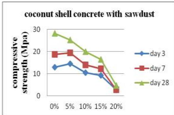
Figure 1: Comparison of CC and CSC with added fibre
