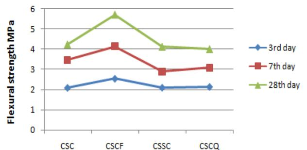
Figure 8: Comparison of CSC, CSSC and CSCQ with addition of fibre
