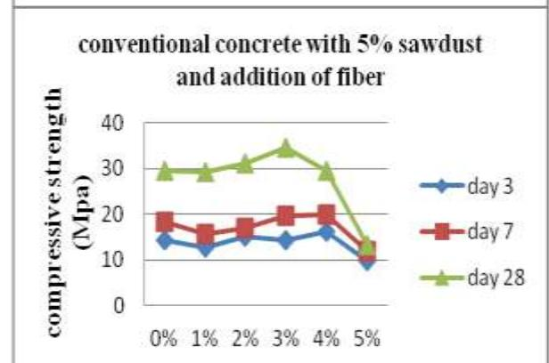
Figure 3: Comparison of CCS and CCQ for 5% sawdust with addition % of fibre
