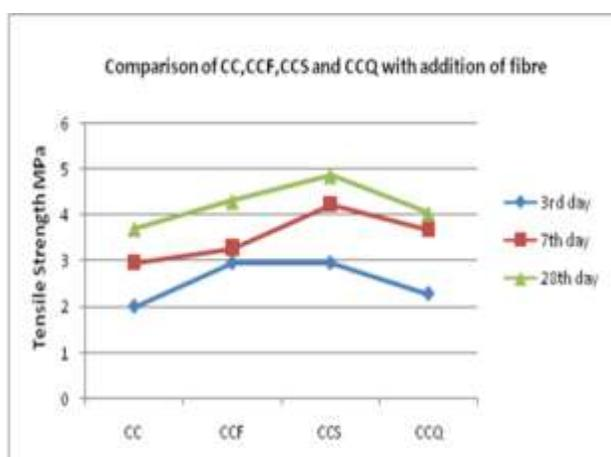
Figure 5: Comparison of CC, CCF, CCS and CCQ with addition of fibre.
