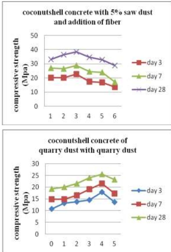
Figure 4: Comparison of CSSC & CSCQ with % of fibre
