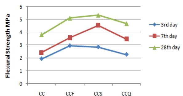
Figure 7: Comparison of CC, CCS and CCQ with addition of fibre
