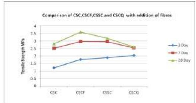
Figure 6: Comparison of CSC, CSCF, CSSC and CSCQ with addition of fibre
