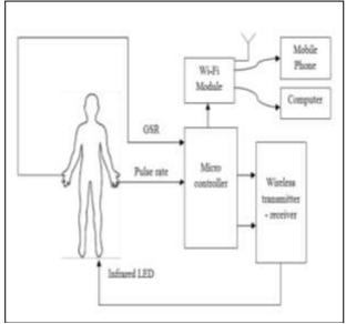
Figure 1: Block diagram of the Stress monitoring and IR therapy prototype
