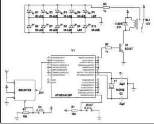
Figure 4: Block Diagram of Therapy unit
