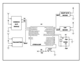
Figure 3: Block Diagram of Sensor circuit
