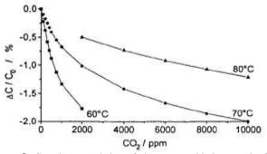
Figure 5: Capacitance variation of the sensor with increase in  $\mathrm{CO}_2$  concentration
