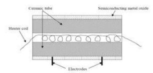
Figure 3: Schematic diagram Taguchi gas sensor
