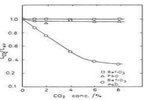
Figure 7: Sensitivity graph of different materials for different  $\mathrm{CO}_2$  concentration
