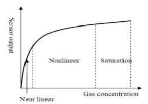
Figure 2: Typical Gas Sensor Output Curve (It Consists Of Near Linear, Nonlinear And Saturation Regions)
