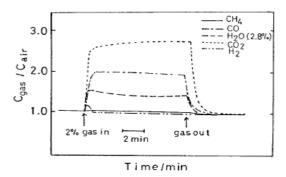
Figure 7: Comparison of sensitivity of equimolar mixture  $CuO-BaTiO_3$  with other gases on exposure to 2%  $CO_2$ .
