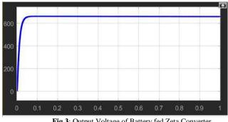
Fig.3: Output Voltage of Battery fed Zeta Converter
