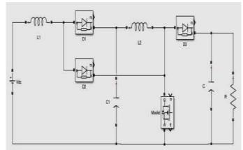
Fig.7: Equivalent Circuit diagram of Cascaded Boost Converter
