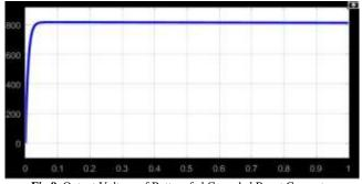
Fig.9: Output Voltage of Battery fed Cascaded Boost Converter
