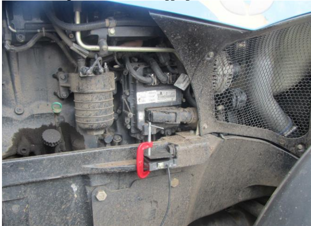
Fig. 7: Installation the sensors (MMA-7260QT) of measuring and recording complex on mobile agricultural machine New Holland T8.390
