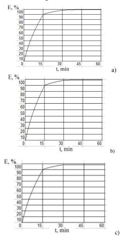
**Fig. 9:** Results of the purification of contaminated water from the technological lubricant by a compositional adsorbent, the granulometric composition of which: a) 0.03 - 0,1 mm; b) 0.1 - 1 mm; c) more than 1 mm.
