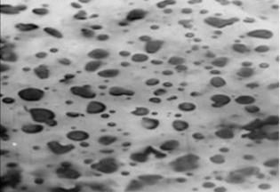
Fig.4: Microstructure of adsorbent from a sunflower husk
