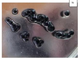
**Fig. 5:** Characteristics of the granulation process: a) - chitosan granules; b) - composite granules of chitosan with modified sunflower husk
