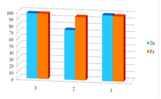
**Fig. 7:** Dependence of the efficiency of cleaning (E) sewage from heavy metal ions by different materials: 1 - chitosan granules; 2 - powder chitosan; 3 - chitosan granules with modified sunflower husk
