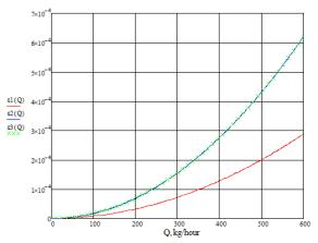
Fig 6: The dependence plot of strain gauge relative strain absolute value on the mass flow rate of air
