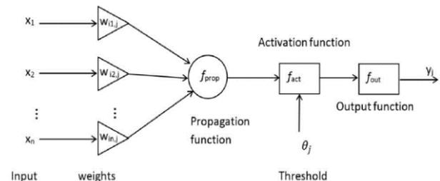
Fig.3: Artificial Neural Network with Activation Function.
