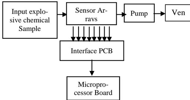
Fig 2: Working of Electronic Nose System
