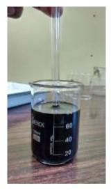
Fig. 2.3:. Stability test with rod penetration
