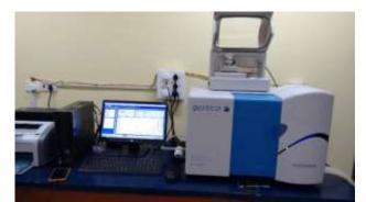
Fig. 2.1: Particle size analysis with PARTICA LA-960
