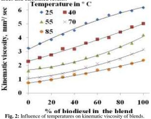
It can be observed from the figure that decease in kinematic viscosity of blends at lower temperature is higher compared to higher temperatures. This may be attributed to decreased resistance of flow at higher temperatures.
