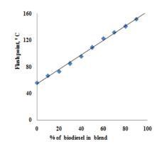
Fig. 3: Influence of volume fraction of biodiesel on flash point of blends.
