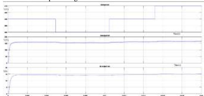
Fig. 12 Input and output of closed loop converter with source variation
