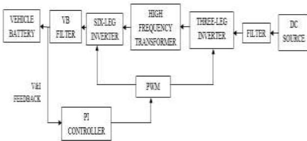
Fig. 3 Block Diagram of Proposed closed loop three phase DC-DC converter
