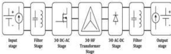
Fig. 1: Block diagram of proposed three phase DC-DC converter
