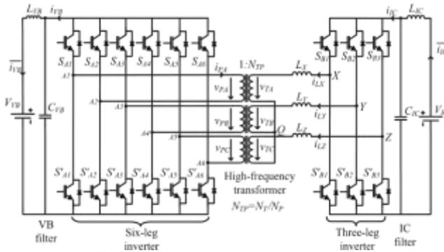
Fig. 2: Three phase six leg DC-DC converter
