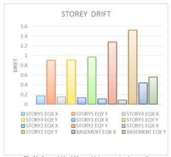
Fig 20: Storey drift of 32 mm thick composite shear wall
