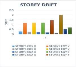
Fig 15: Storey drift of 32 mm thick Steel Plate shear wall
