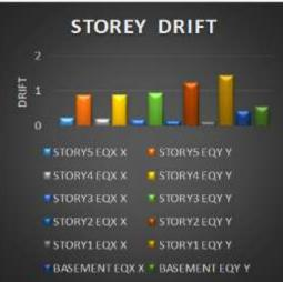
Fig 7: Storey drift of 225 mm thick RCC shear wall.
