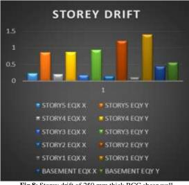
Fig 8: Storey drift of 250 mm thick RCC shear wall
