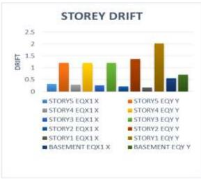
Fig 11: Storey drift of 24 mm thick Steel Plate shear wall
