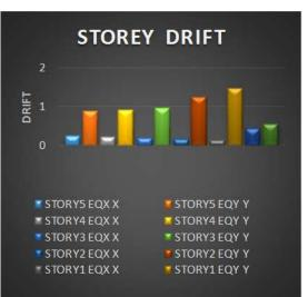
Fig 6:: Storey drift of 200 mm thick RCC shear wall
