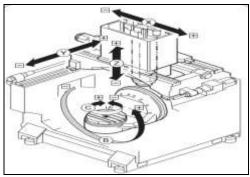
Fig. 1: Five - Axis Machining Center setup.
