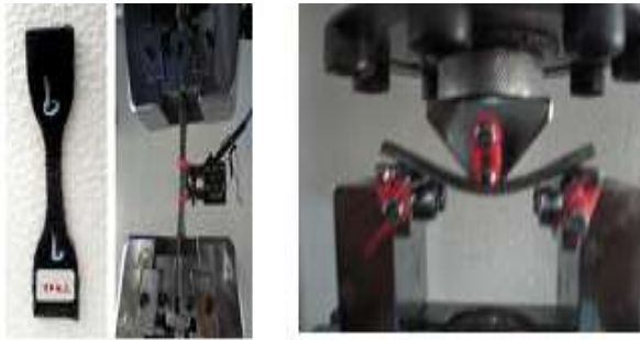
Fig. 5: Tensile and Flexural Testing of composite
