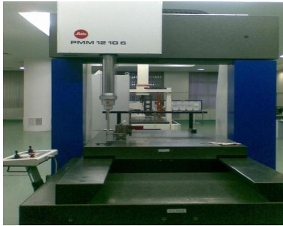
Fig. 1: 3D Coordinate Measuring Machine.
