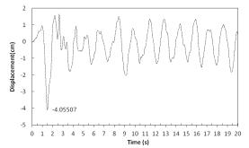
Diagram 20: Displacement of Upper Level of Tank in Fullness State of 100% in Case there is Damper in Middle Level under Chi-Chi Earthquake
