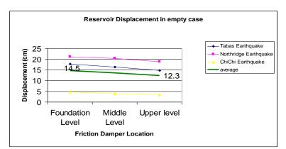
Diagram 30: Displacement of Upper Level of Empty Tank for Different Positions of Damper
