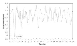
Diagram 21: Displacement of Upper Level of Tank in Fullness State Of 100% in Case there is Damper in Upper Level under Chi-Chi Earthquake
