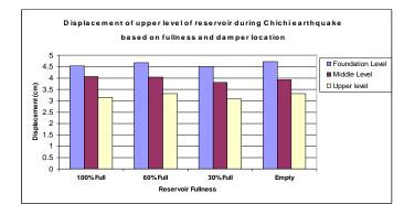
Diagram 33: Displacement of Upper Level of Tank Based on Position of Damper for Different States in Chi-Chi Earthquake
