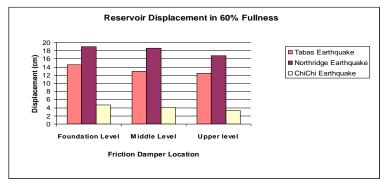
Diagram 25: Displacement of Upper Level of Tank in Fullness State Of 60% for Different Positions of Damper
