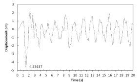
Diagram 19: Displacement of Upper Level of Tank in Fullness State Of 100% in Case There Is Damper in Foundation Level under Chi-Chi Earthquake
