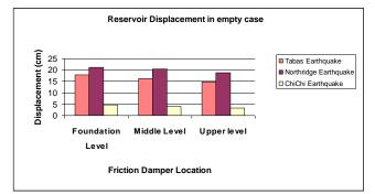
Diagram 29: Displacement of Upper Level of Empty Tank for Different Positions of Damper
