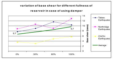
Diagram 35: Variations of Base Shear in Different States of Tank with Damper
