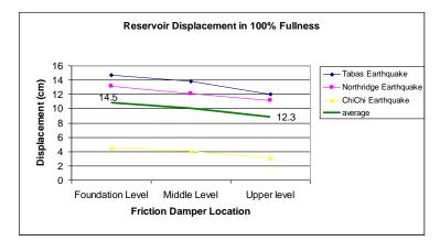
Diagram 24: Displacement of Upper Level of Tank in Fullness State of 100% for Different Positions of Damper
