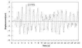
Diagram 4: Displacement of Upper Level of Tank in Fullness State of 100% under Chi-Chi Earthquake
