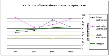
Diagram 34: Variations of Base Shear in Different States of Tank without Damper
