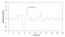
Diagram 12: Displacement of Upper Level of Tank in Fullness State Of 100% in Case There Is Damper in Middle Level under Tabas Earthquake
