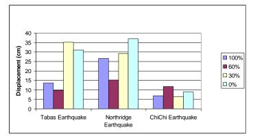
Diagram 9: Comparing Displacement of Upper Level of Tank in Empty Tank under the Studied Earthquakes
