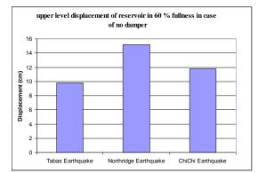
Diagram 6: Comparing Displacement of Upper Level of Tank in Fullness State Of 60% under the Studied Earthquakes
