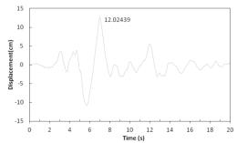
Diagram 13: Displacement of Upper Level of Tank in Fullness State Of 100% in Case There Is Damper in Upper Level under Tabas Earthquake
