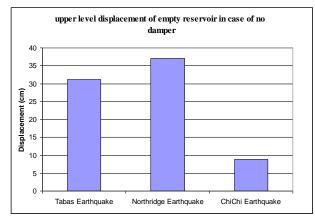
Diagram 8: Comparing Displacement of Upper Level of Tank in Empty Tank under the Studied Earthquakes
