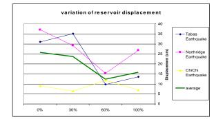
Diagram 10: Comparing Displacement of Upper Level of Tank in Empty Tank under the Studied Earthquakes
