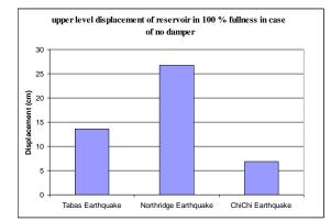
Diagram 5: Comparing Displacement of Upper Level of Tank in Fullness State Of 100% under the Studied Earthquakes
