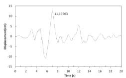
Diagram 17: Displacement of Upper Level of Tank in Fullness State of 100% in Case There Is Damper in Upper Level under Northridge Earthquake
