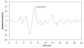
Diagram 11: Displacement of Upper Level of Tank in Fullness State Of 100% in Case There Is Damper in Foundation Level under Tabas Earthquake
