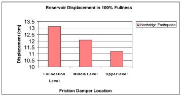
Diagram 18: Displacement of Upper Level of Tank in Fullness state of 100% For Different Positions of Damper under Northridge Earthquake
