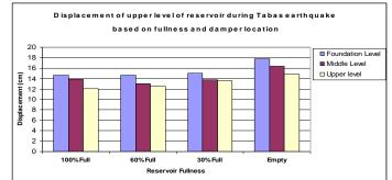
Diagram 31: Displacement of Upper Level of Tank Based on Position of Damper for Different States in Tabas Earthquake
