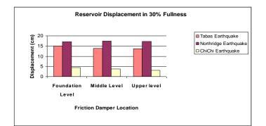
Diagram 27: Displacement of Upper Level of Tank in Fullness State Of 30% for Different Positions of Damper
