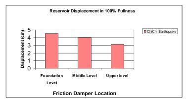
Diagram 22: Displacement of Upper Level of Tank in Fullness state of 100% For Different Positions of Damper under Chi-Chi Earthquake
