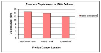
Diagram 13: Displacement of Upper Level of Tank in Fullness State of 100% for Different Positions of Damper under Tabas Earthquake
