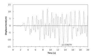
Diagram 2: Displacement of Upper Level of Tank in Fullness State Of 100% under Tabas Earthquake
