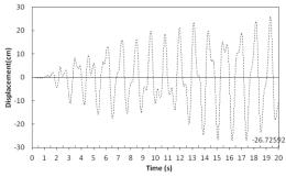
Diagram 3: Displacement of Upper Level of Tank in Fullness State of 100% under Northridge Earthquake
