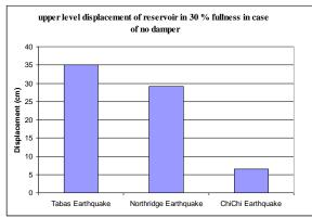
Diagram 7: Comparing Displacement of Upper Level of Tank in Fullness State Of 30% under the Studied Earthquakes
