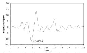
Diagram 16: Displacement of Upper Level of Tank in Fullness State of 100% in Case There Is Damper in Foundation Level under Northridge Earthquake
