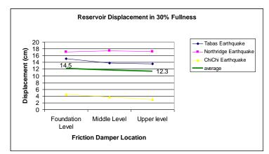
Diagram 28: Displacement of Upper Level of Tank in Fullness State Of 30% for Different Positions of Damper
