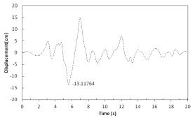
Diagram 15: Displacement of Upper Level of Tank in Fullness State of 100% in Case There Is Damper In Foundation Level under Northridge Earthquake
