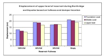
Diagram 32: Displacement of Upper Level of Tank Based on Position of Damper for Different States in Northridge Earthquake
