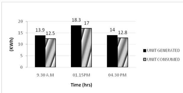
**Fig.8.** Unit Generation and Consumption Per Day
