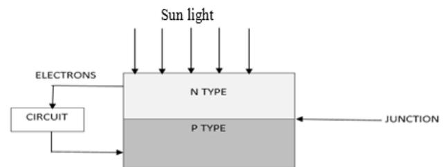
Fig. 1. Transection of Solar Cell
