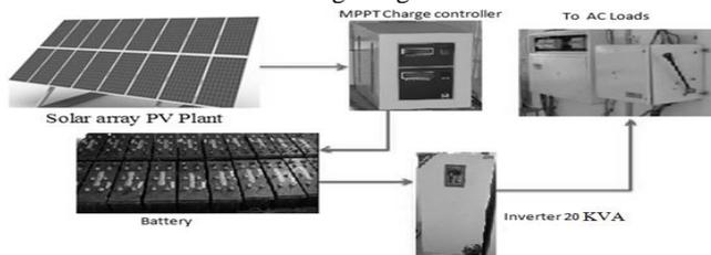
Fig.2. 15 KW off grid SPV Plant
