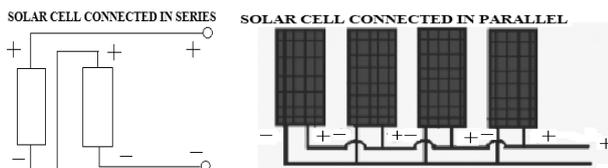
Fig.3. Solar cell in series & parallel connection
