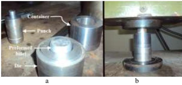
Figure 7: a- Preparing the preformed billet inside the die, b- the process of pressing
