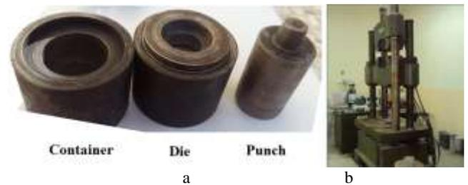
**Figure 5:** a- parts of die, b- hydraulic pressing machine
