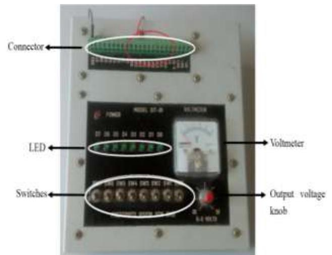
Fig. 2: Muscle part of the learning tool - testbox as simple testing tool
