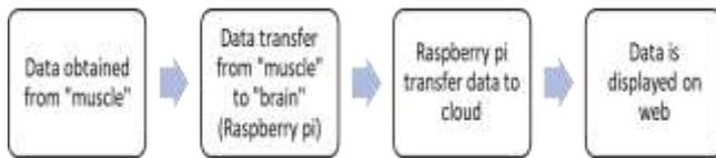
**Fig. 6:** Flow chart on data transmission from “muscle” to “brain” to “cloud”
