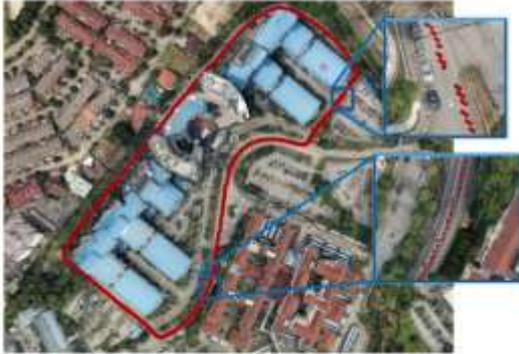
**Fig. 4:** The map shows the actual GPS coordinates collected during experiment. Shown inset is the magnified view, highlighting the GPS precision's problem, where the point is not precisely on the path travelled by the vehicle. The problem is more apparent near tall buildings and trees
