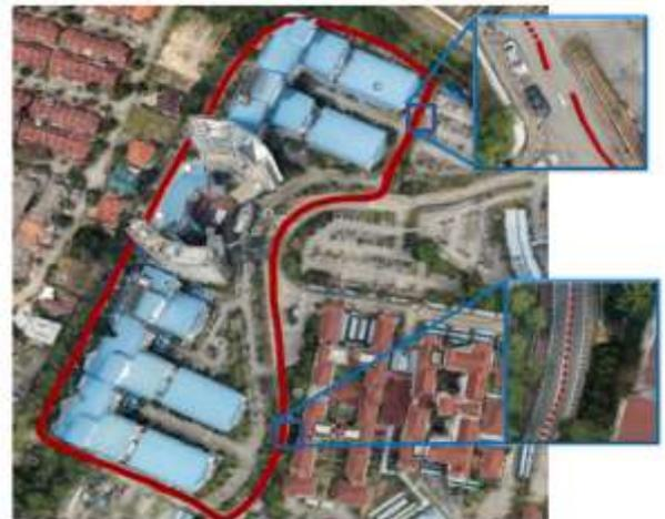
**Fig. 12:** The map shows the improved GPS coordinates points from our proposed method. Inset images show that the problem of imprecision with GPS sensor readings now has been significantly reduced
