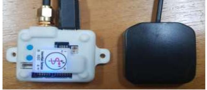
**Fig. 1:** The InertialSense® uAHRS miniature attitude heading reference system module (on the left) used for inertial measurement, and InertialSense® miniature magnetic mount GPS/GLONASS Antenna (on the right) used in GPS data collection for distance estimation
