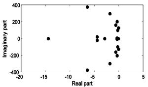
Fig. 7: Location of eigenvalues in complex plane with optimal PSS parameters
