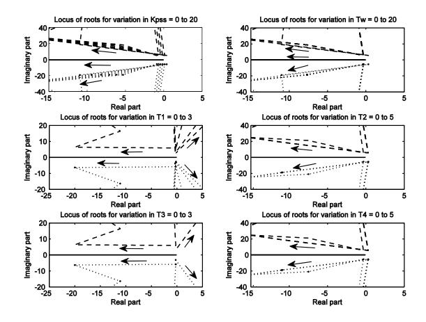
Fig. 4: Movement of the eigenvalues with the variation of PSS parameters
