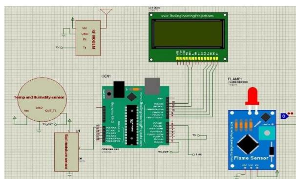
Fig. 7: Proteus Model of One Sensor Node in Agricultural Field.
