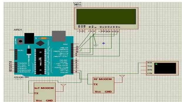
Fig. 8: Proteus Model of Collector-Zigbee-Node MCU and Cloud Server/Mobile App.
