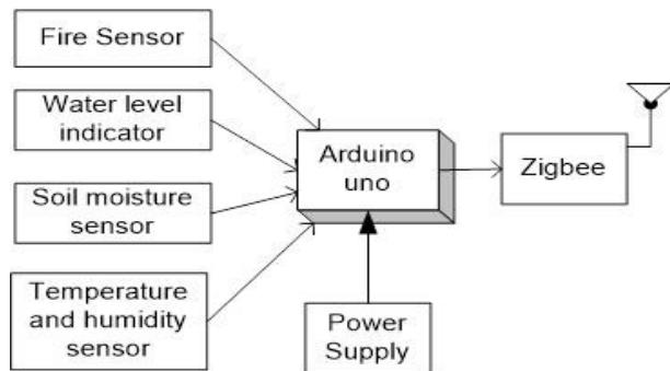
Fig. 5: Architecture of One Node Using Zigbee.
