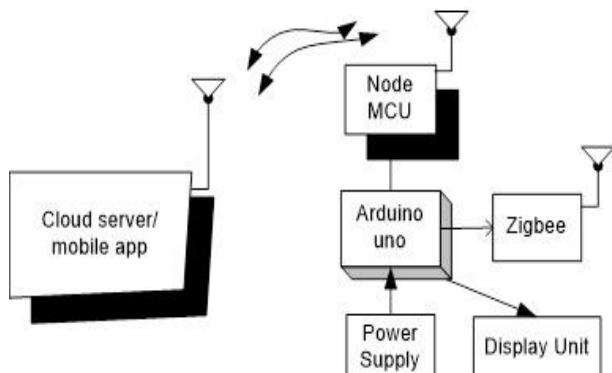
Fig. 6: Architecture of Collector-ZigBee-Node MCU and Cloud Server/Mobile App.
