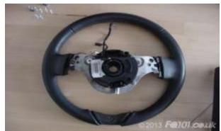
Fig. 1: Steering Wheel with Angle Sensor.
