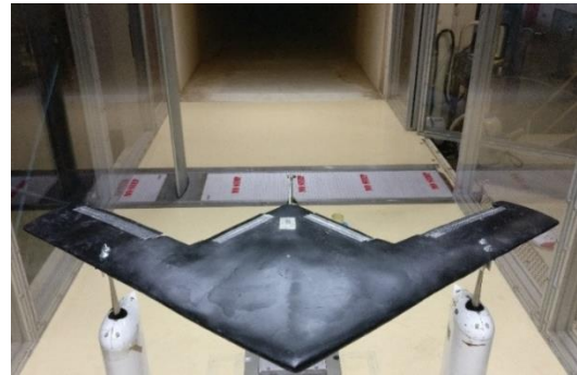
Fig. 7: Finalized position of model inside wind tunnel
