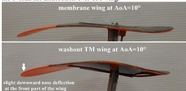
Fig. 10: Downward nose deflection at the front part of TM wing
