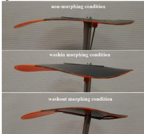
Fig. 1: Washin and washout morphing wing
