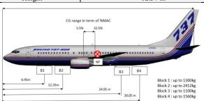
Fig. 4: Weight and position for block
