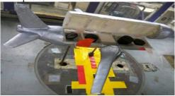
Fig. 8: Weights inside the aircraft model
