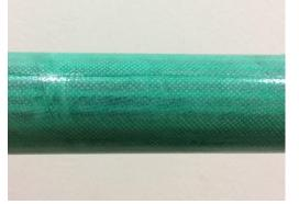
Fig. 6: Resin fully capsulate the preform
