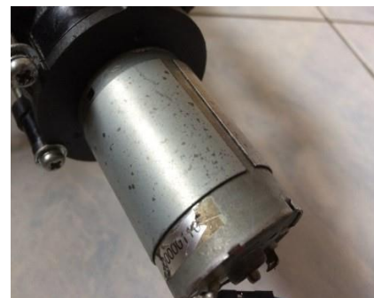
Figure 4: 12 V DC motor
