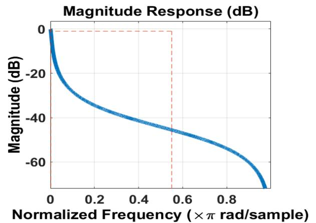
Fig. 3: Magnitude Response of the Filter.
