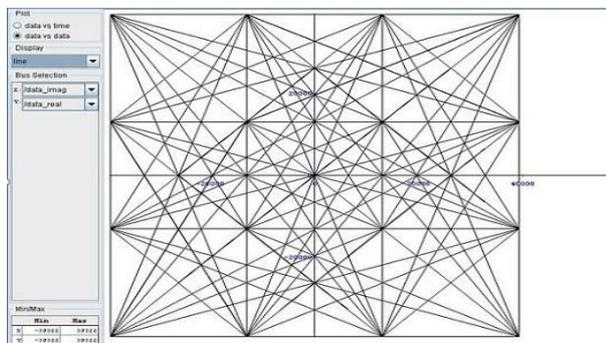
Fig. 9: AGC Input 16-QAM Constellation on Hardware in Chipscope Bus Plot.
