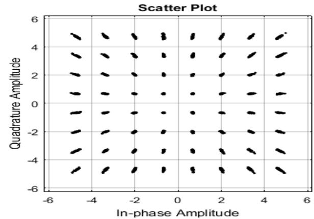
Fig. 7: A) Constellation Plot: Proposed Digital AGC Output for A 64-QAM Signal.
