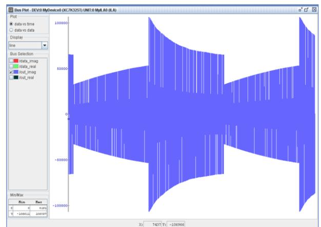
Fig. 12: AGC Output Signal on Hardware in Chip Scope Bus Plot in Data v/s Time Mode.
