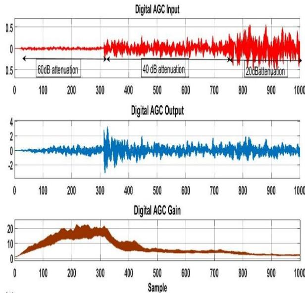
Fig. 5: Transient Response of AGC with 16-QAM-OFDM Signal.
