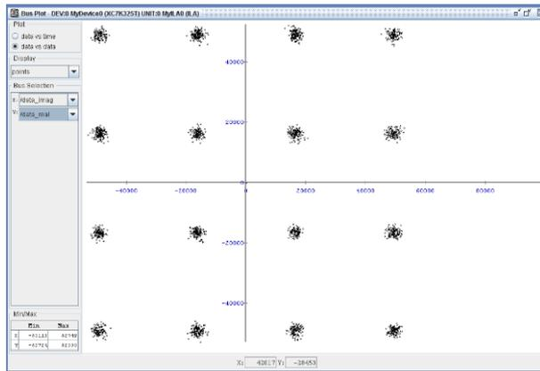
**Fig. 14:** AGC Output 16-QAM Constellation with SNR 20 Db on Hardware in Chip Scope Bus Plot in Data v/s Data Mode.
