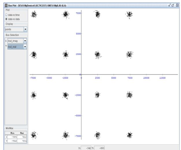
Fig. 13: AGC Output 16-QAM Constellation with SNR 20 Db on Hardware in Chip Scope Bus Plot in Data v/s Data Mode.
