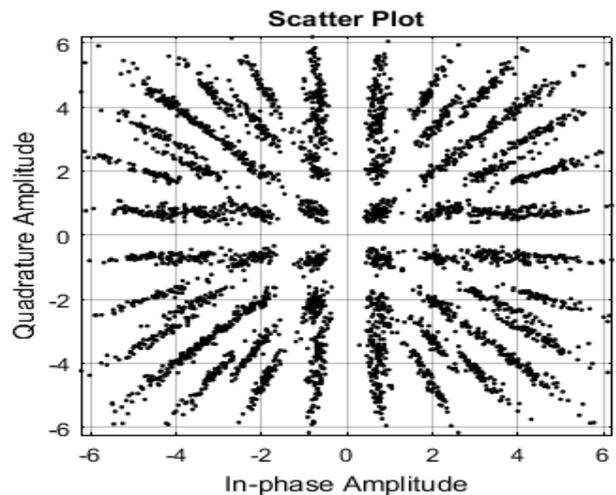
Fig. 7: B) Constellation Plot: Conventional Digital AGC Output for A 64-QAM Signal.
