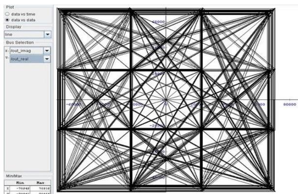
Fig. 10: AGC Output 16-QAM Constellation on Hardware in Chip Scope Bus Plot.
