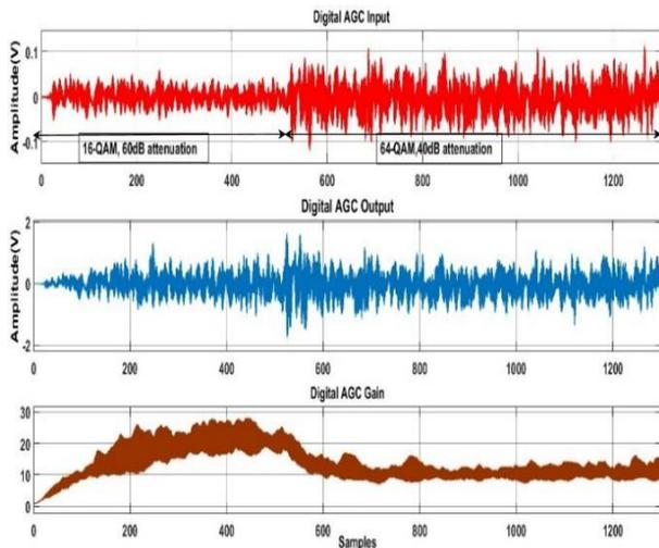
Fig. 8: Transient Response of the AGC for Adaptive Modulation-Based Signal.
