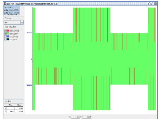
Fig. 11: AGC Input Signal on Hardware in Chip Scope Bus Plot in Data V/S Time Mode.
