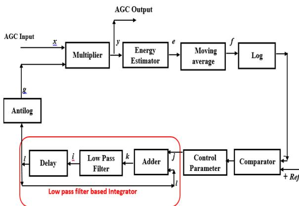
Fig. 2: Proposed Architecture of Proposed Digital AGC for WLAN Architecture.
