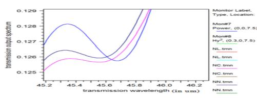
Figure 8: Graphical representation of relative wavelength shift versus output power for normal cell.
