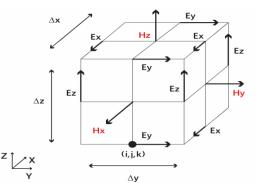
Figure2: An yee cell in 3 dimensional plane corresponding to magnetic field computation.
