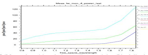
Fig 12: Represents the transmission wavelength spectrum with respect to extinction coefficient of gold metal
