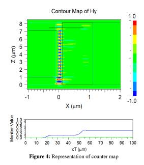
Excitation along the interface is depicted in the figure 4, with x axis as length and the z axis as breadth and the colour-bar towards right side represents the instantaneous values of power. Along with this the monitor power values along the sensing layer of the device is shown just below the contour map.
