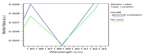
Figure 11: Represents the transmission wavelength shift for the normalised cell and abnormal cell (Cytoplasm).
