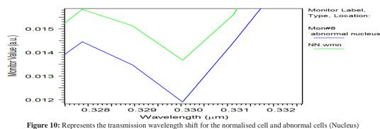
The graph 10 represents the transmission wavelength shift spectrum of normal and abnormal cell nuclei. In the previous case we case it is observed that the shifts in the wavelength due the differences between the dielectric properties of the normal and abnormal cell varies by 2000 nm/RIU.
