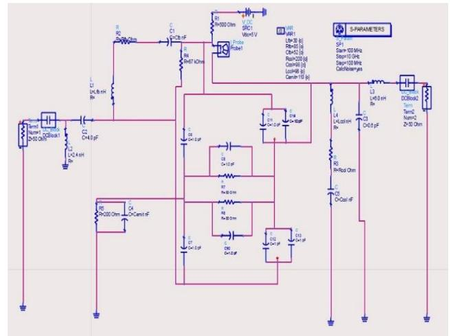
Fig. 4: Cylindrical Surrounding Double-Gate MOSFET Based LNA.
