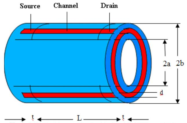
Fig. 3: Cylindrical Surrounding Double-Gate MOSFET model [17].
