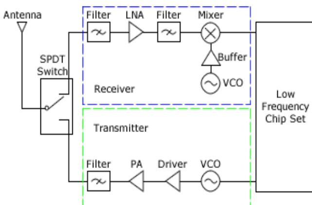
Fig. 1: Block Diagram of a Communication System with an LNA [5].
