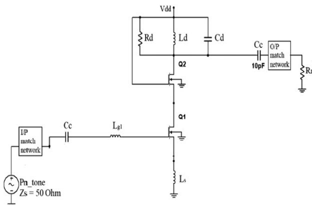
Fig. 2: Conventional MOSFET LNA with feedback [16].
