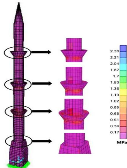
Fig. 21: Normal and Shear Stress Distribution of 76.2 M Minaret.
