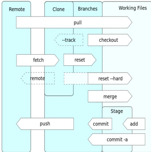
**Fig.7** : Some data flows and storage levels in the Git revision control system
