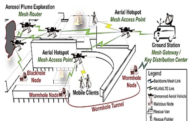
Fig. 1. Example of a deployment scenario of UAV-WMN and two routing attacks in disaster relief.
