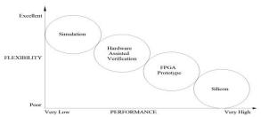
Fig.1: Trade-off between the flexibility and performance of various verification methods.
